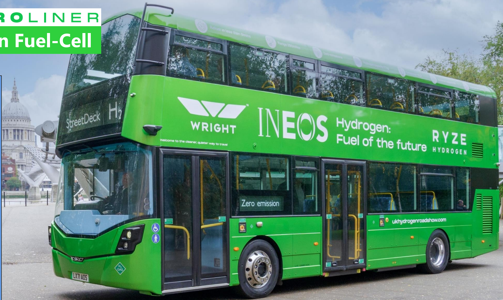
World's first production Hydrogen Double-Deck Bus, designed and built in Ballymena, NI.
